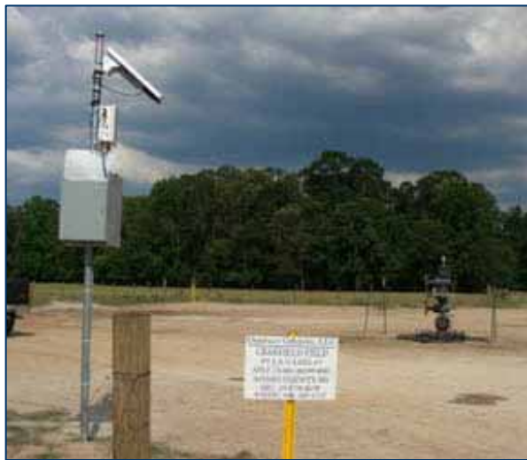
Satellite uplink of real-time data is transmitted every 10 seconds to researchers at The University of Texas at Austin for monitoring and analysis.
